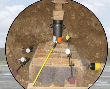
In Situ Direct Shear Test
